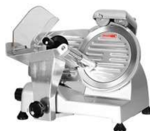
AS-250B Meat Slicer (250 mm) Size: 575x465x415 mm Thickness: 0.2~12 mm, Width: 180 mm Power: 150 w
