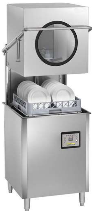
HS-50 Commercial Dishwasher Washing Time: 60~300 s Cap.: 50 Baskets/H Rinse Temp.: 85~90 c Tank Size : 42 Ltrs. Warmer Volume: 28 Ltrs. Size: 675 x 740 x 1375 mm Power: 9 Kw~380 ~415 v
