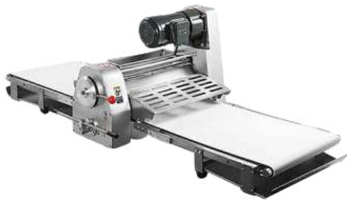
TSP 520 Dough Sheeter Table Top Outline Size: 2400×920×650 mm Conveyer Belt Size: 500×1980 mm Roller Range: 1~35 mm Power: 550 w
