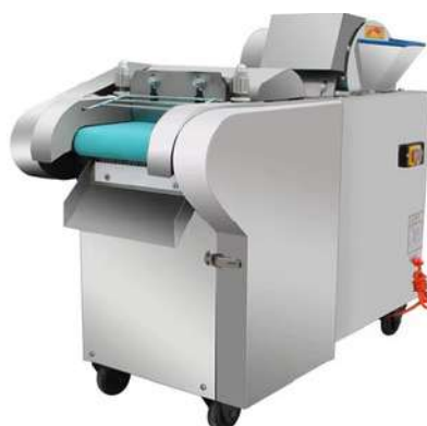
Model: 660 Conveyor vegetable cutting machine with Machine Head Dicing Machine Production Cap: 100-300 kg/h Slice Thickness: 1-6mm adjustable Cut Size: 2-23 mm Tool Holder Raised Dimension: 30 mm Size: 880*430*750 mm Voltage : 220 V Power: 0.75 kw
