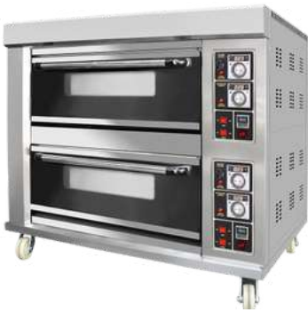
GBO-24 Bakery Gas 2 Deck 4 Tray Oven Size: 1300x890x1410 mm Chamber: 870x650x230 mm Tray Size: 400x600x30 mm Power: 200 w
