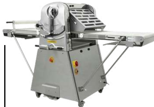
E 520 Dough Sheeter Standing Outline Size: 2550×1000×128 mm Conveyer Belt Size: 500×1980 mm Roller Range: 1~45 mm Power: 750 w
