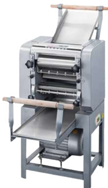
Model No:- MT 60 Commercial Noodle Machine Roll Parameters :- \phi 89 \times 220 Power:- 1.5 kw
